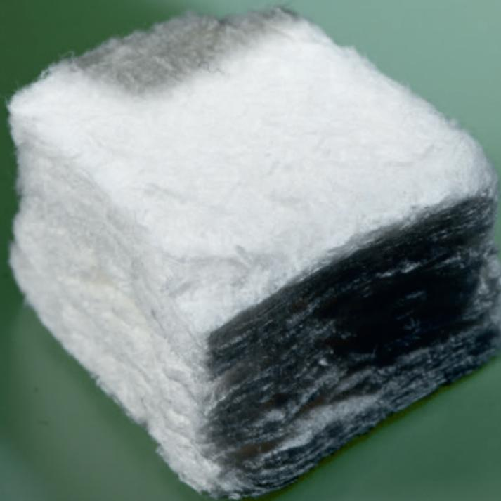
Foam made from cellulose fibres that can be used as a substitute for polystyrene foam, for example.
